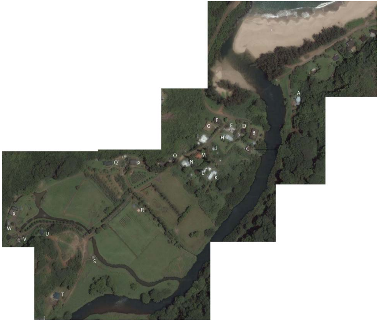
Figure 3: Aerial imagery of terrain along western bank of lagoon. Buildings labeled A-X were surveyed for ground elevation and building height above the ground.
