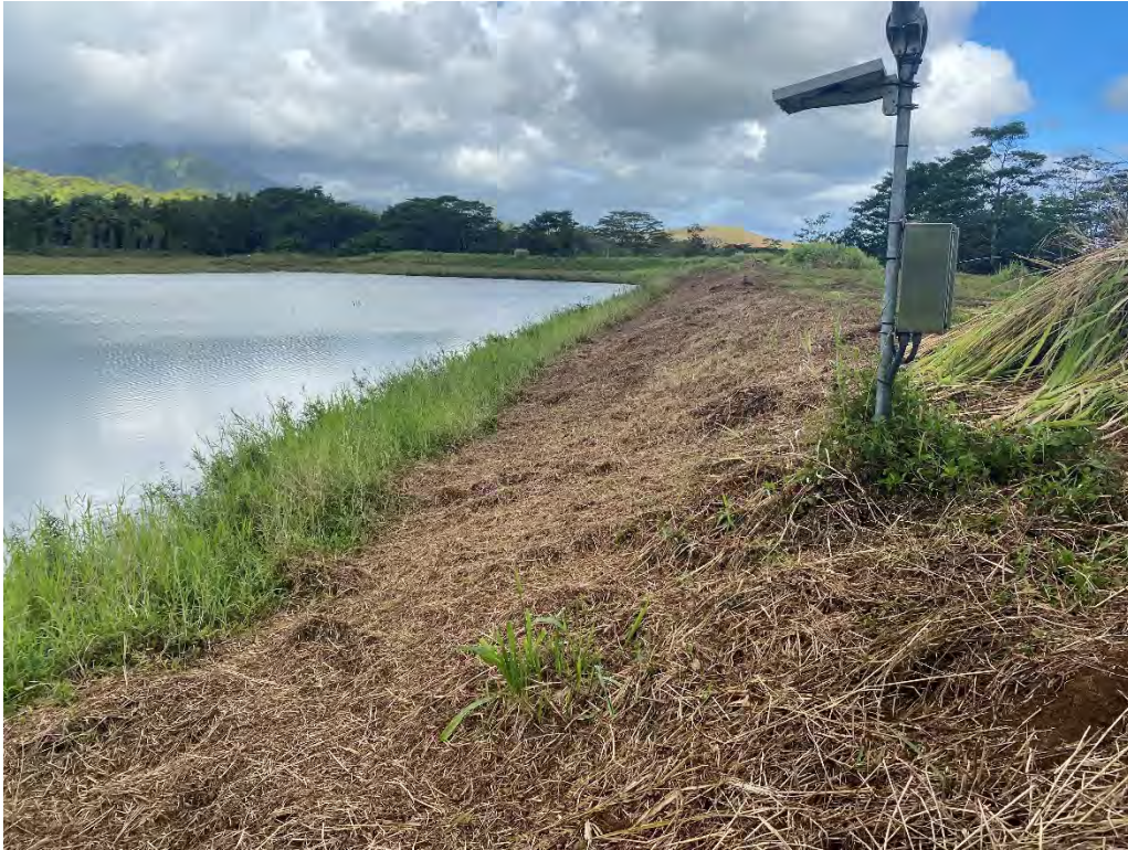
Photo B-41: Digital Reservoir Gage (upstream shoulder of embankment crest near right abutment of right embankment segment)
